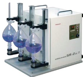
SR-2DS with Separatory funnel shaking platform (Option)
