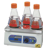
Shake-XR *Dedicated for Figure 8 (Page 54) 3 pcs of 500mL Erlenmeyer flask Various options
