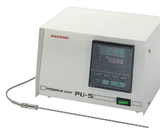
Can temperature program control with an optional program unit.
